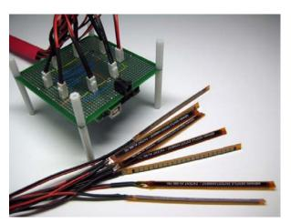
Fig. 6. Bending Sensors Attached to the Arduino.
