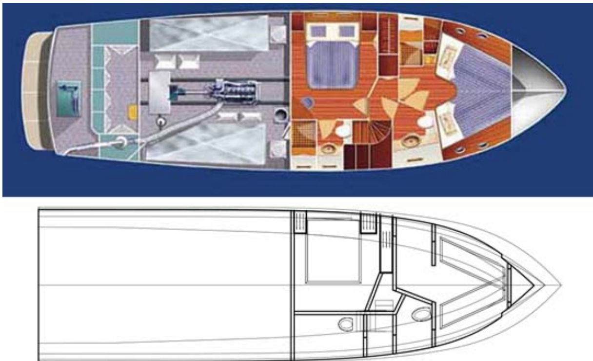
Fig. 12 Selene 49 lower deck layout alternative 2 and the model comparison [URL-3]
