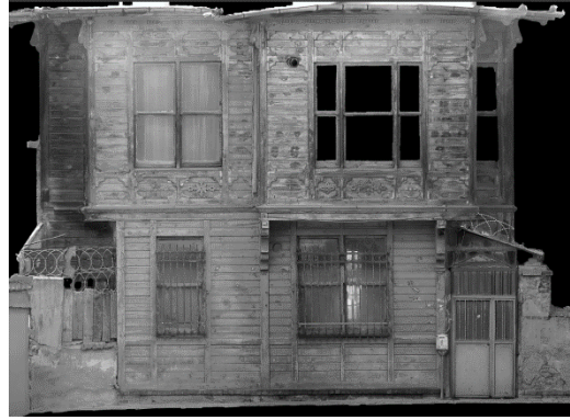
Figure 7. High resolution orthophoto of 3D textured model produced with a point cloud and external camera support (source: Alper Yiğitoğlu)
