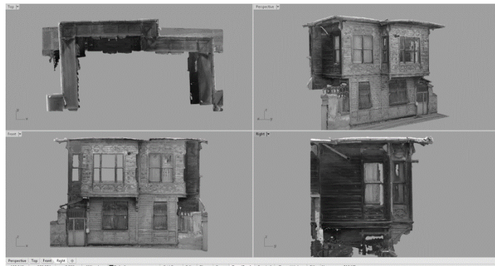
Figure 6. Screen view of 3D textured model produced with a point cloud and external camera support (source: Alper Yiğitoğlu)
