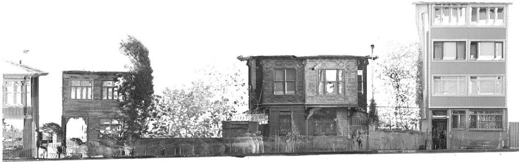
Figure 5. Orthophoto from a 3D point cloud (source: İlyas Keskin and Nazım Keskin, student at Istanbul Medipol University Vocational School of Architectural Restoration)
