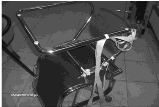
Figure 5 Connection of electrical cables to strain gages
