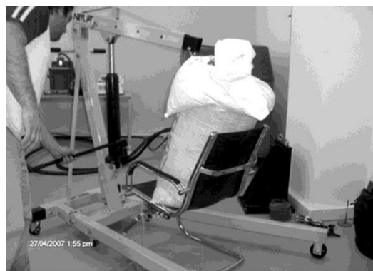
Figure 8 120 kg load on backside of the chair 2nd and 3rd measurements
