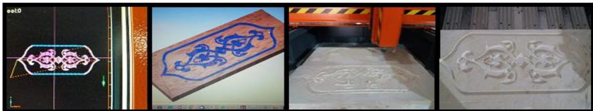
Figure 14: Modeling and processing in Cnc router in Artcam 2012 program
